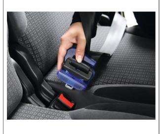
The Securiseat is a safety device for the exclusive use of disabled persons who are at risk of inappropriate behaviour during transport. Prevents seat belts from being accidentally unfastened. Once the Securiseat is locked, the seat belt cannot be removed except with the keys provided or a car key.
