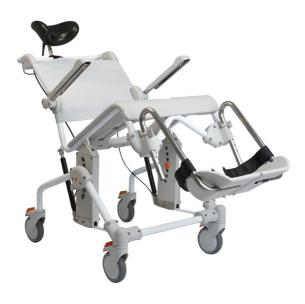
can be moved to the back and also to the sides. The seat tilts from 0 to -35° (or +5 to -30° by a simple adjustment). The seat height can be adjusted without tools from 34 to 46.5 cm. Removable seat for easy cleaning.
