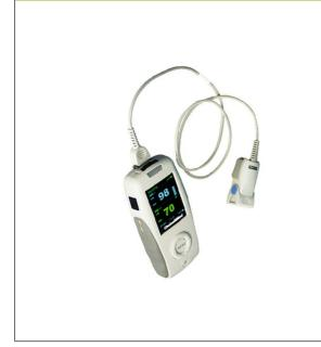
Interchangeable SpO2 sensor for use on adult and paediatric patients. Visual and audible alarms : SpO2, PR, sensor disconnected, low battery. Automatic shut-off. Two-colour OLED display showing SpO2%, heart rate, pulse bar graph, plethysmogram. Supplied with one adult sensor. Operates with 2 AA batteries.
