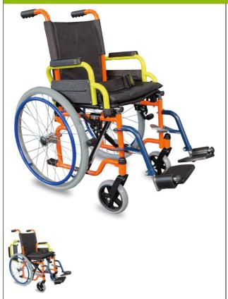
This manual wheelchair is designed for children. Folding, it features folding armrests, a fixed seat, and folding footrests. The rear wheels are 51 cm (20") in diameter and have handrails and brakes. The front wheels are smaller, with a diameter of 15 cm. A seat belt is integrated to ensure better support for the user.
