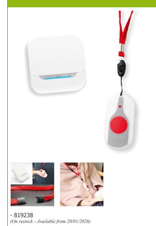
Alarm system consisting of a transmitter to be worn as a pendant with a call button and a receiver that plays an alert sound. The receiver, plugged into the mains, has 4 volume levels from 25 to 110 dB and 36 melodies. Range: 100 m. When the person in bed presses the button, the receiver goes off instantly. CR2032 battery supplied with transmitter.
